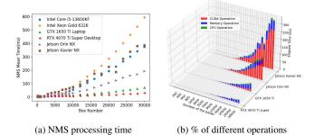
Figure 3. System effects of latency attacks. a) # objects vs. NMS processing time on heterogeneous computing devices; b) percentage of GPU CUDA, memory transfer and CPU logic operations on embedded and desktop GPUs.
