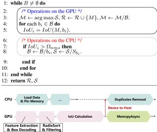
Figure 2. Interactions between GPU-CPU in the NMS.
