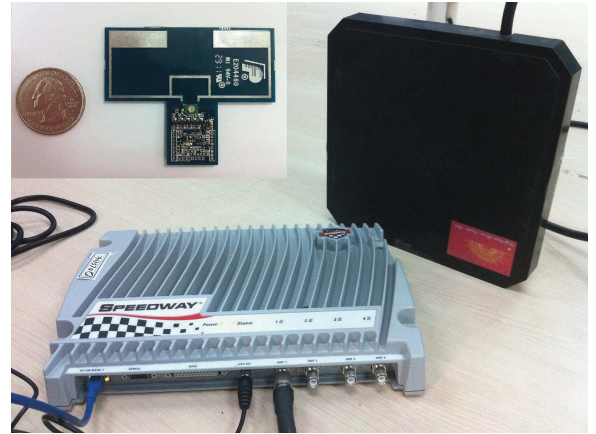
Fig. 6. Antenna-reshaped WISP Tag and Reader
