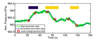
Figure 10: Data processing for level change detection.
