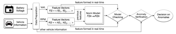
Fig. 9: B-Diag detects (and verifies) the anomalies in engine RPM based on battery voltage with an online data-driven model.
