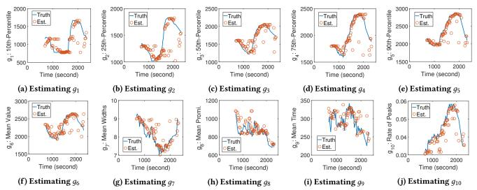
Fig. 13: Estimating the features of engine RPM based on those of battery voltage, with the traces in Fig. 6 as an example.
