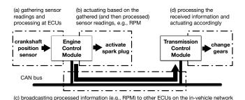
Fig. 1: Vehicle's cyber operations: gathering, processing, transmitting information and actuating accordingly.
