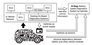
Fig. 2: B-Diag diagnoses vehicles with a cyber-physical approach by exploiting automotive batteries as sensors.
