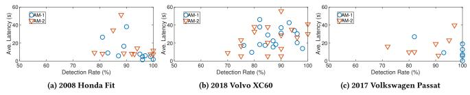
Fig. 38: B-Diag detects the anomalies of Honda Fit, Volvo XC60, and Volkswagen Passat with averaged rate/latency of  $\{92\%, 88\%, 96\%\}/\{91\%, 86\%, 87\%\}$  and  $\{11, 26, 12\}/\{15, 28, 18\}$ s, with the two anomaly models of AM-1 and AM-2, respectively.
