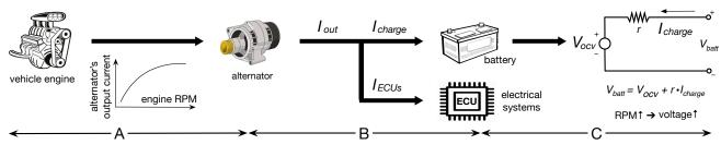
Fig. 5: Other things being equal, a faster engine RPM leads to a higher battery voltage.
