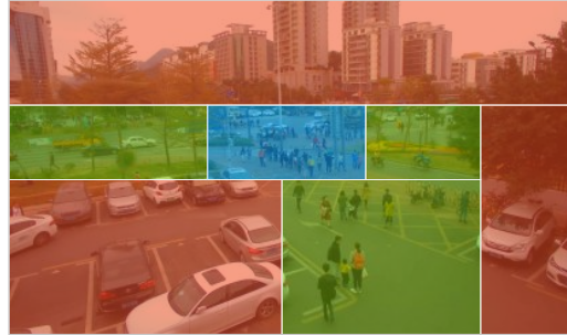
Figure 1: An illustration of REMIX for pedestrian detection in a 4K image. For the blue block in the middle, an expensive network is applied due to the high density of objects. Networks of medium sizes are used in green blocks. Red blocks are processed using cheap networks or even skipped.
