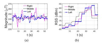
Fig. 26. The variation of signals in different sections along the same passage. (a) Geo-magnetic signal; (b) WiFi signal.
