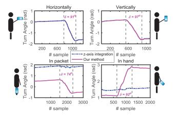
Fig. 5. The detection of turn angles with our method and integrating of gyroscope's z-axis readings without any preprocessing.
