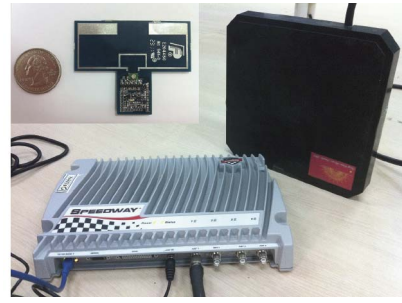
Fig. 8. Antenna-reshaped WISP tag and reader.
